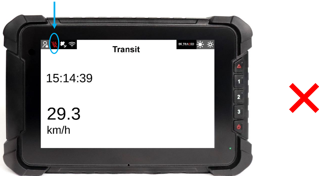
Figure 2 - Red power indicator light: device not powered
