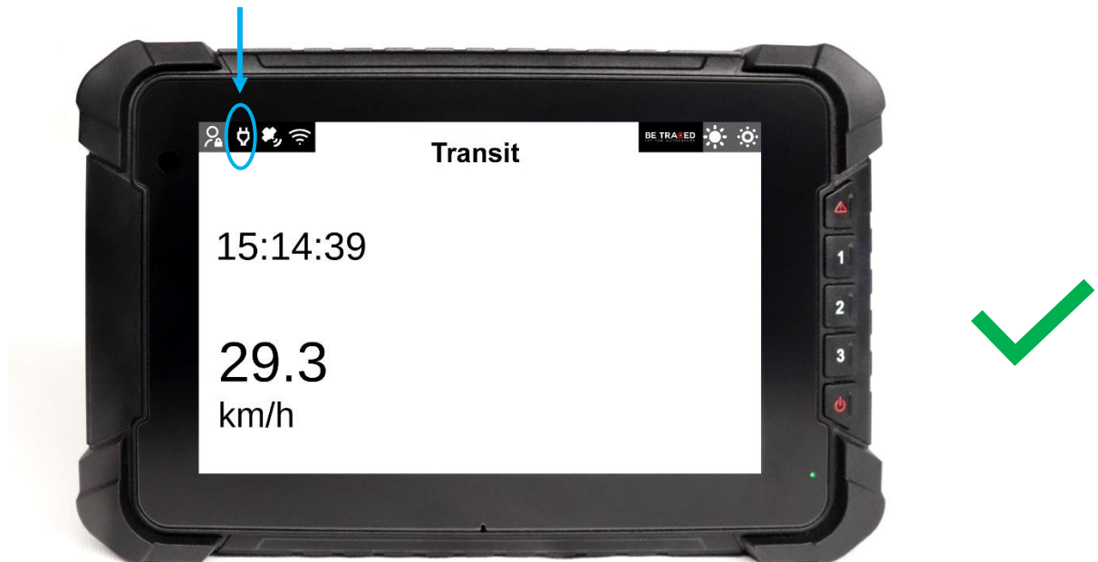
Figure 1 - White power light: device powered correctly
